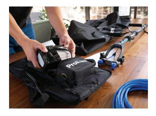
STEP 1: Unpack battery charger, found in the white box within the shipping container, and insert into the battery pouch on the backpack.
