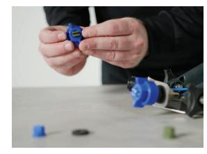
**STEP 2:** Push spray tip out of lock nozzle cap and replace with desired spray tips. Place sprayer tips in first, followed by the rubber washer.
