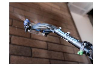
**STEP 3:** When sprayer is first turned on after connection, expect a few seconds for the motor to draw liquid for maximum spray.
