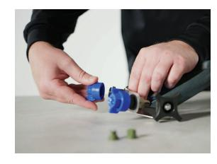
STEP 1: Twist lock nozzle cap counterclockwise. Handle with care, so as not to misplace spray tip and rubber washer.
